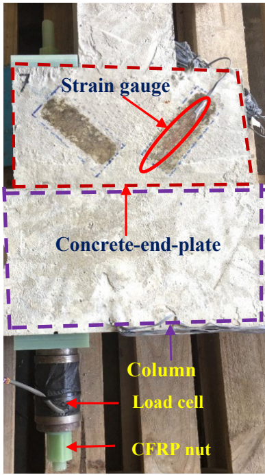
Fig. 3. Details of strain gauges and load cells.
