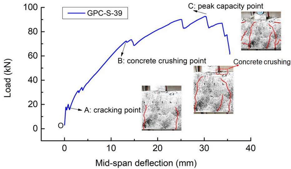
**Fig. 6.** Load-deflection curve of the tested beam under quasi-static load
