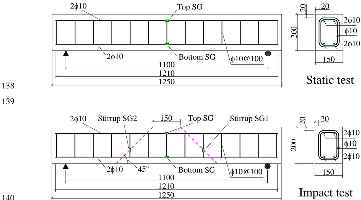
141 **Fig. 2.** Configuration of the tested beams and locations of strain gauges
