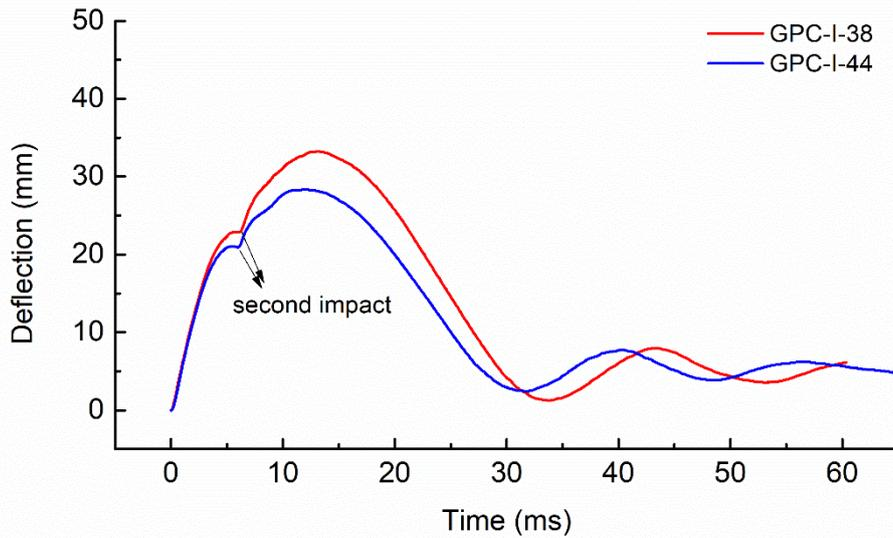
**Fig. 12.** Displacement time histories of the tested beams
