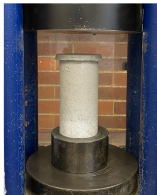
Fig. 2. Set-up of quasi-static compressive tests.
