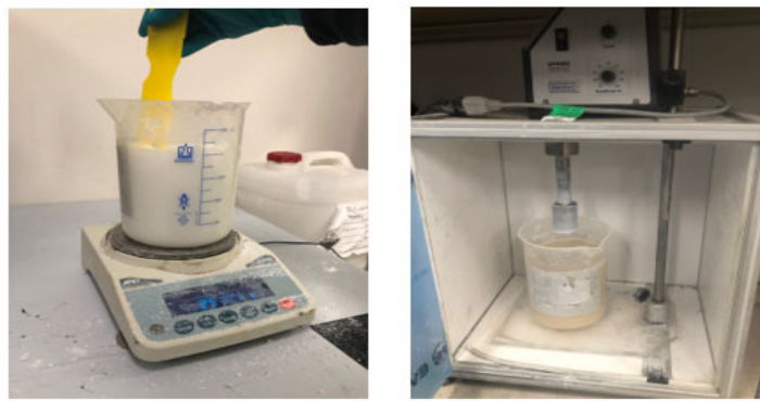
Fig. 1. Ultrasonic mixing of nano silica
