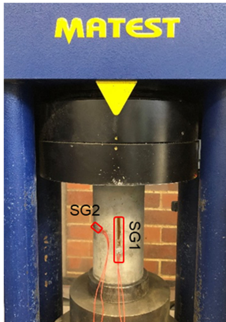
154 155 Fig. 2: Quasi-static compressive test setup (SG: strain gauge).
