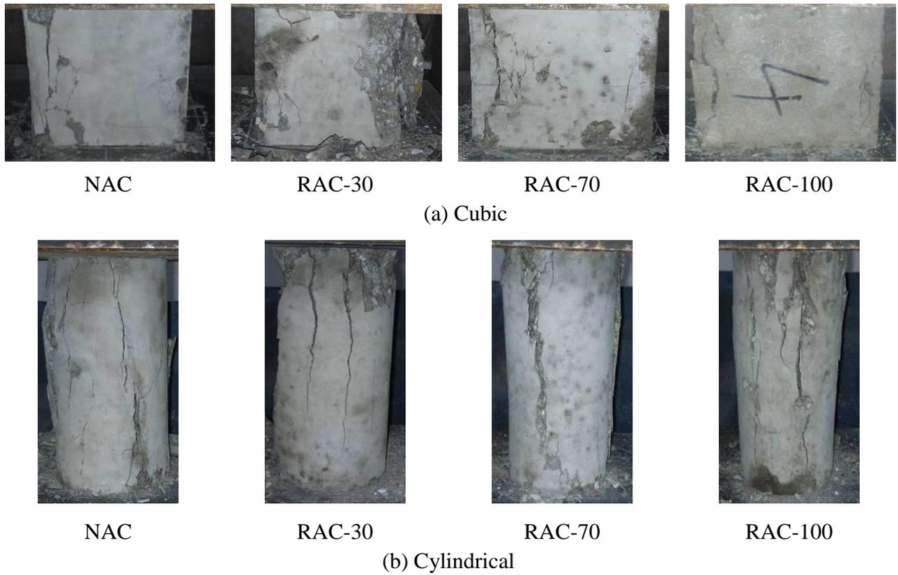
Fig. 1 Failure modes of specimens under quasi-static test
