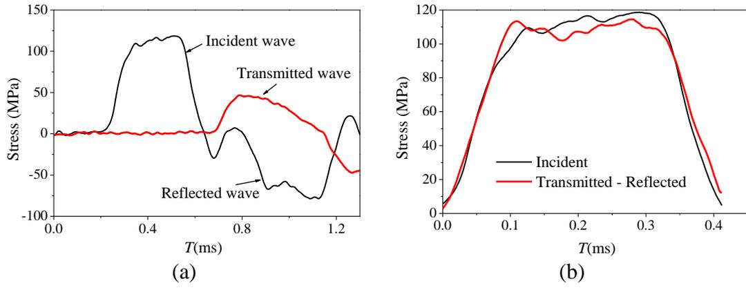
Fig. 6 Typical impulse waves of SHPB test
