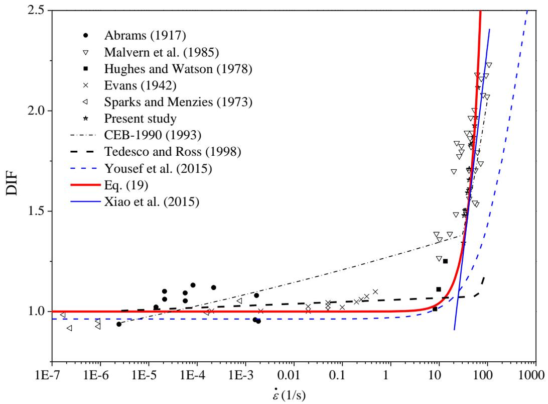
Fig. 10 DIF - strain rate curve for natural concrete
