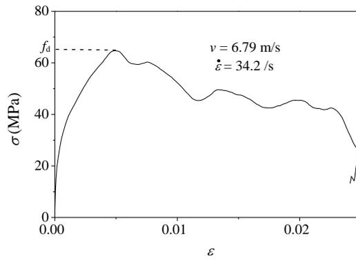
Fig. 7 Typical dynamic stress - strain curve of SHPB specimen
