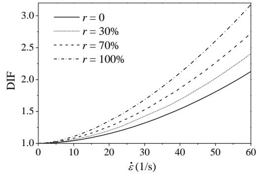
(a) Dynamic compressive strength - strain rate
