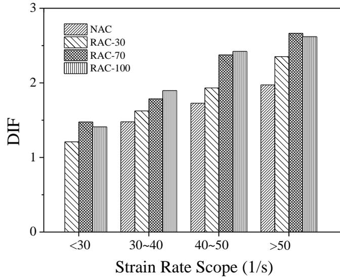
Fig. 9 DIF - strain rate scope
