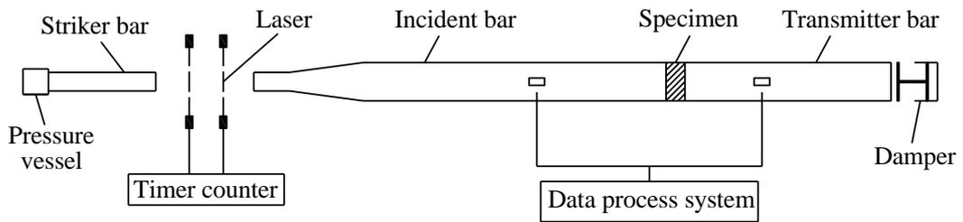
(b) Schematic diagram of SHPB
