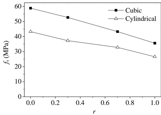
Fig. 2 Quasi-static compressive strength with various RCA replacement percentages
