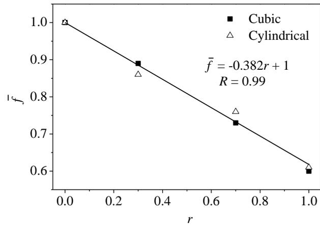
Fig. 3 Normalized quasi-static compressive strength with various RCA replacement percentages
