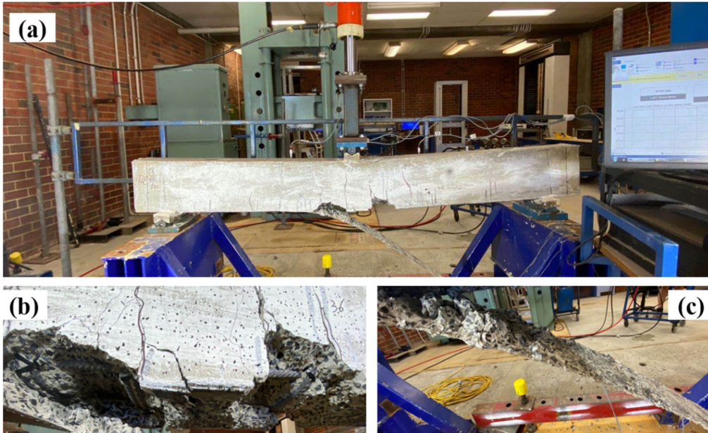
247 248 Figure 14. (a) Failure mode of Specimen BP_16_60; (b) Concrete cracking after debonding; (c) 249 Debonded BFRP sheets.
