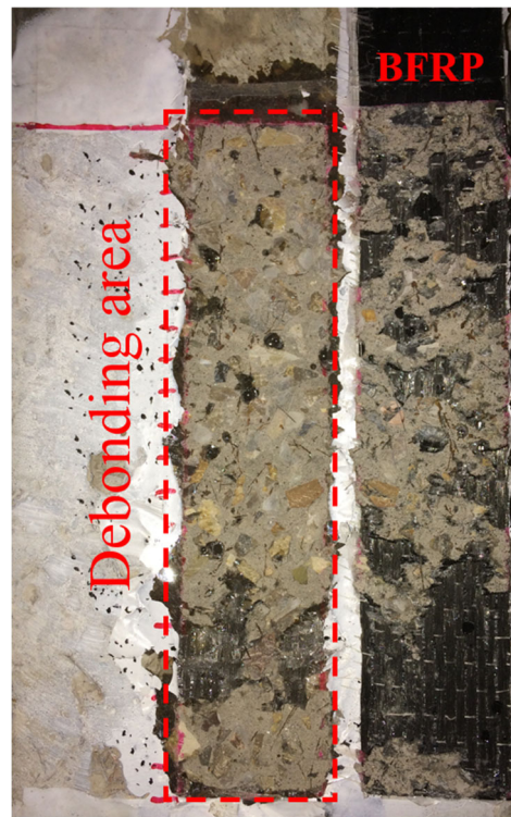
(e) Failure mode of (L) QS1-1 and (R) D1-8-1
