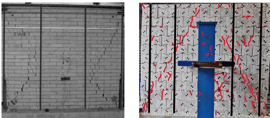
a) The conventional masonry wall [56] b) The interlocking brick wall
