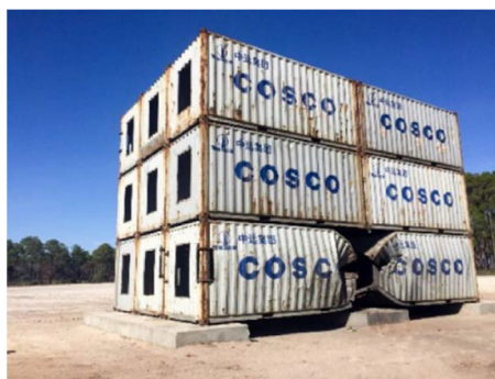
Figure 3. Field test on CONEX for progressive collapse [93].
