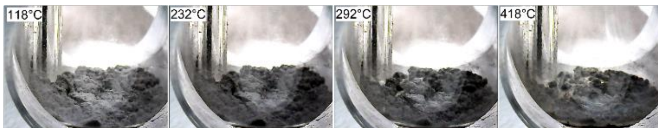
Figure 4: TPPA of 6KAlH 4 -Al 2 S 3 heated under an initial H 2 pressure of 4 bar ( \Delta T/\Delta t = 5 °C/min).
