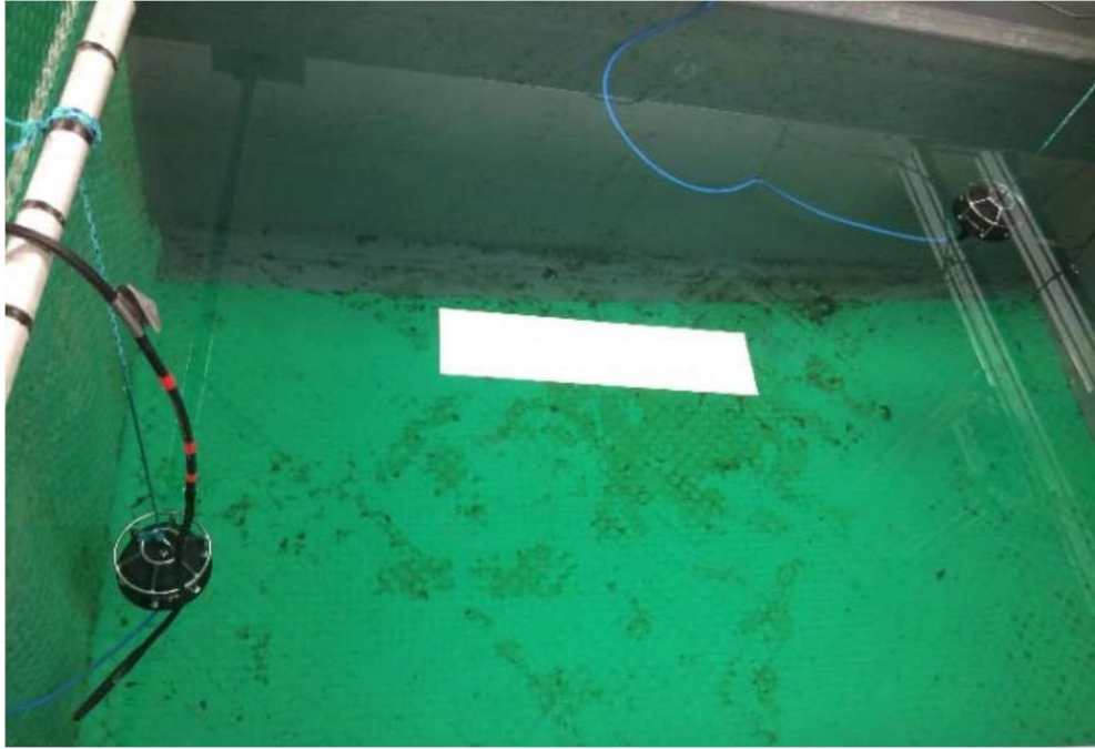
Figure 12: Location of the transducers and hydrophones for forward and feedback links.
