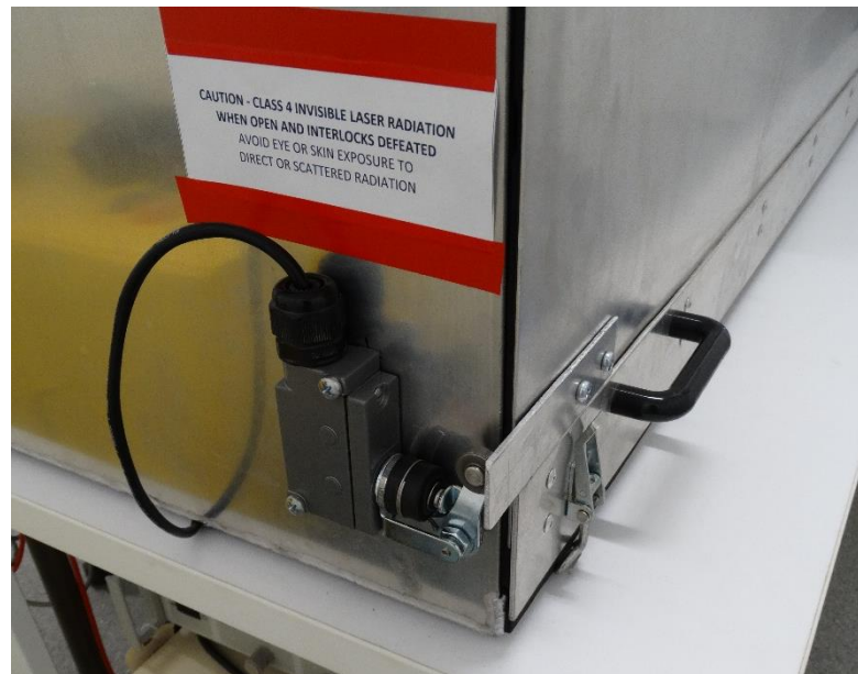
Figure B2. More close-up photograph of the switches that will trigger the interlock system when defeated.
