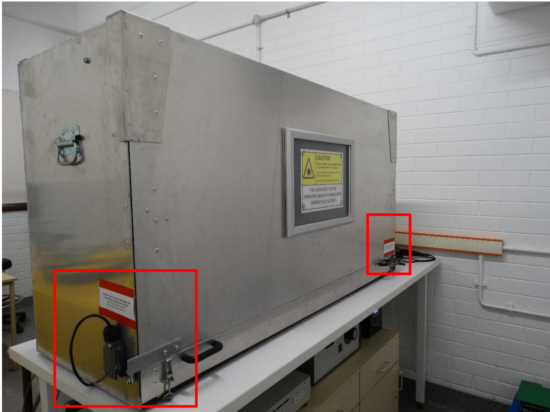
Figure B1. Photographs of the aluminium enclosure when closed. The switches that will trigger the interlock system are inside the red squares.
