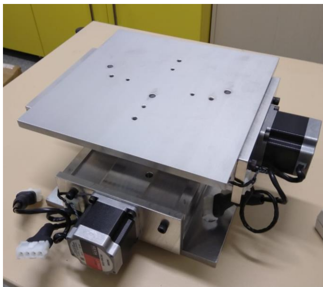
Figure A2. Photograph of the top plate of the motorised positioning table.
