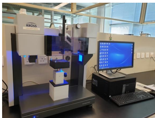
Figure 4.19. Drop shape analyser used for the purpose of this study
