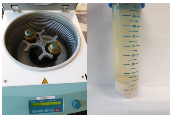
Figure 3.13: Protein precipitation obtained from centrifuge
