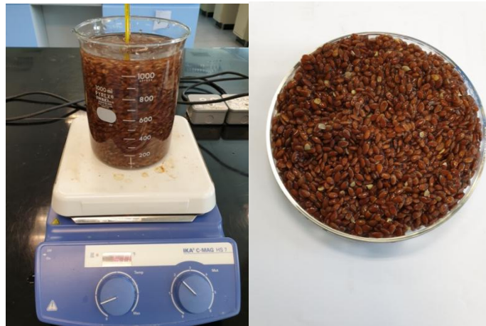
Figure 3.10: Demucilaged flaxseed obtained based on the procedure used
