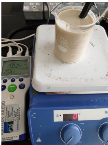
Figure 3.14: Neutralization of protein solution
