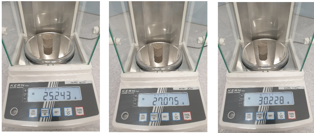
Figure 5.11: weighting of the shale samples
