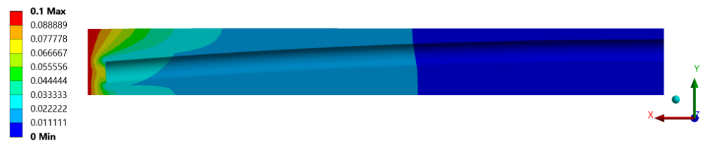
Figure 5. Displacements in SWCNT-reinforced composite.
