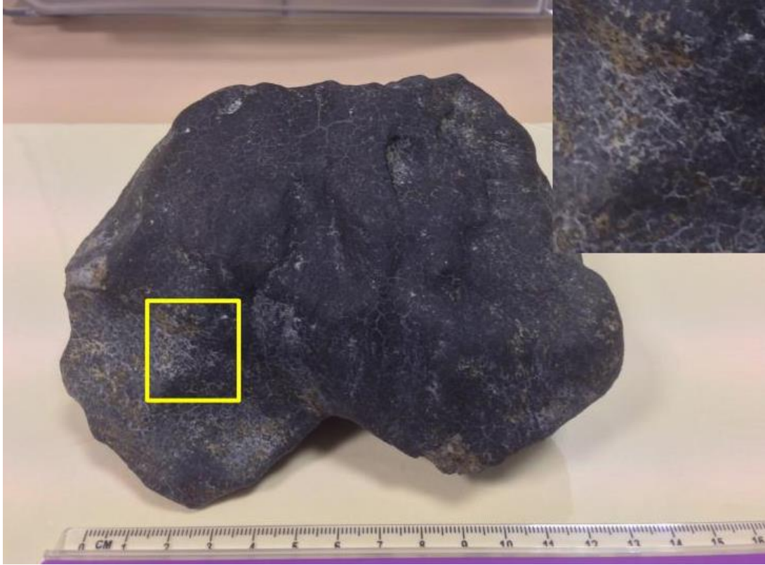
Figure 3. Full mass of the Murrili meteorite – ruler scale is cm. Inset shows close up of fusion crust texture – cracks are infilled with what is most likely lake sediments.
