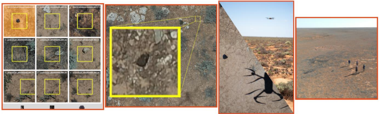
Figure 3. The four stage process for eliminating false positives and verifying meteorite candidates. (From Left to Right) 1) Grid GUI. 2) Zoom-pan GUI. 3) Drone visit. 4) In-person visit.
