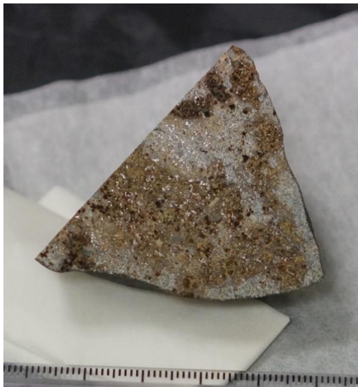
Figure 4. The Wedge used for He pycnometry, magnetic susceptibility and \mu CT scans.
