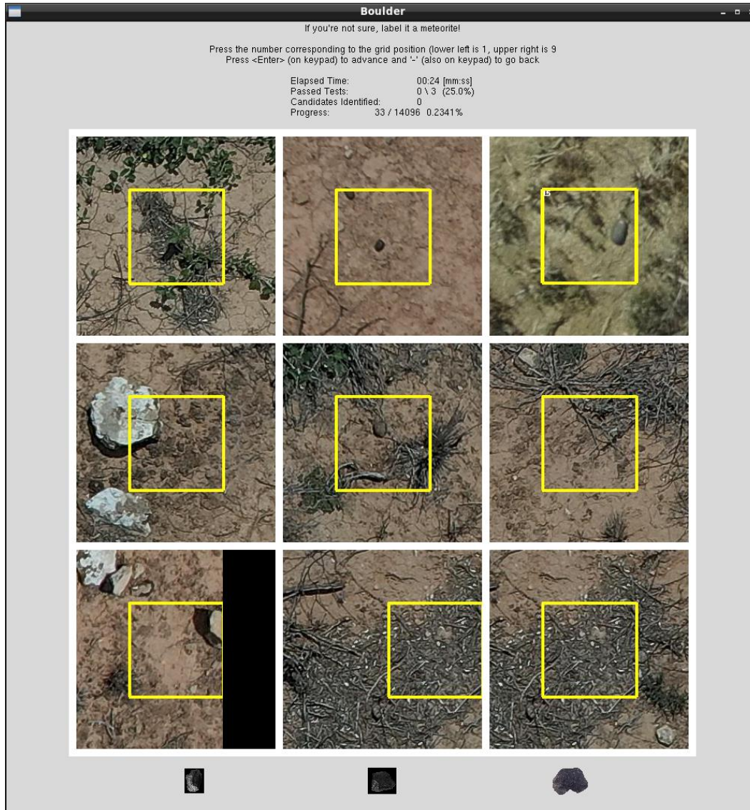
Figure 1. The grid sorting GUI, that allows users a first pass at the model detections. The typical dimensions for the field of view (for each detection) was 67 x 67 cm.
