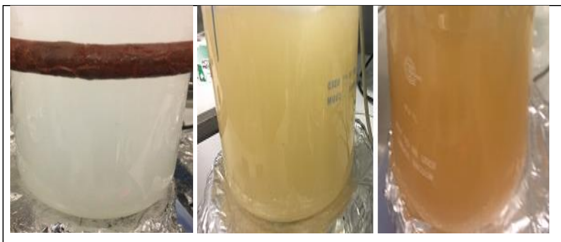
Figure 4-5: Experimental solution at start of experiment (left) and after 2 days with MEG degradation at 90 °C (middle) and 135 °C (right).
