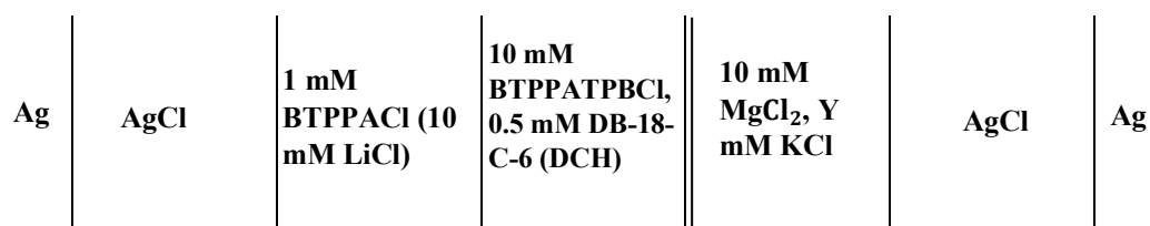
Figure 2.3 The electrochemical cell composition (Y mM is concentration of KCl).
