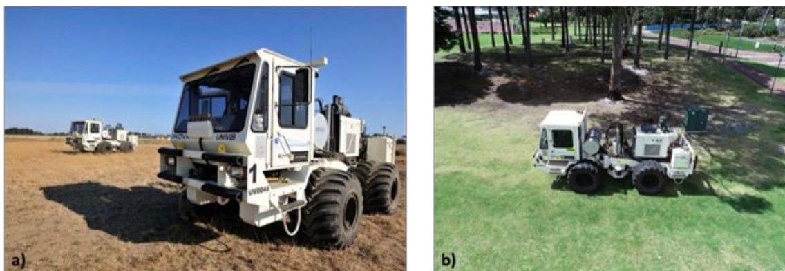
Figure 1. Photos of vibroseis truck at Otway (a), and close to NGL facility (b). Notice different soil conditions at the two sites. Sandy-clay soil at Otway is hard when dry and soft when wet, while sandy soil at NGL is less susceptible to moisture.
