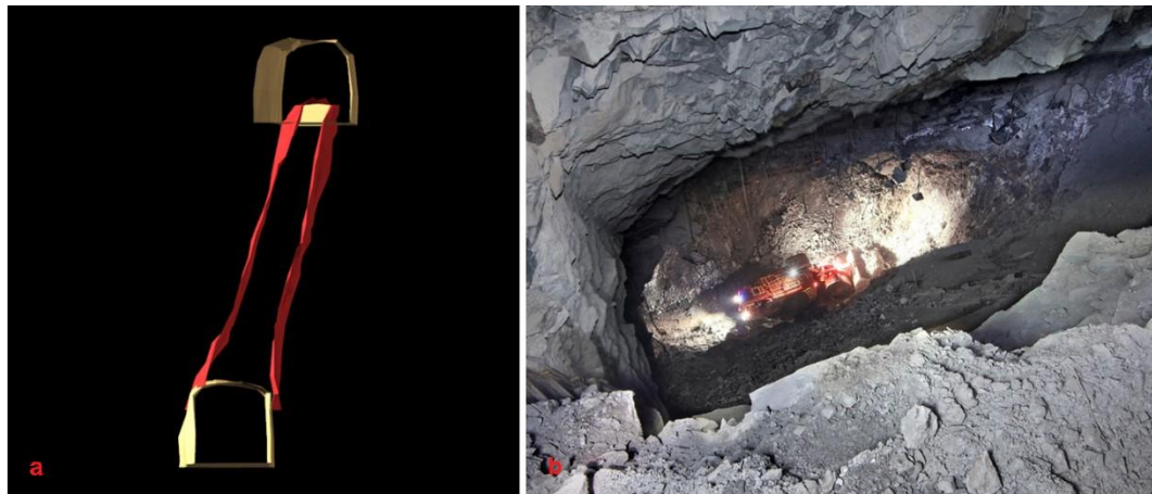
Figure 7-7: Actual stope between two drives: (a) stope scanned by CMS (b) view from upper drive.
