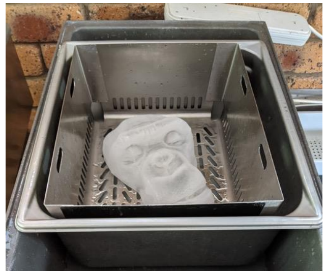
Figure 12. Print after curing process. Image by Gregor Macgregor, 2021.
