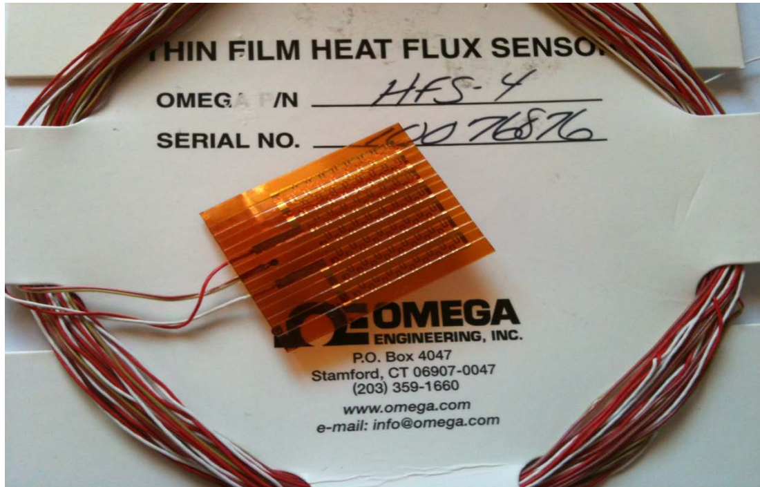
Figure 3.11 Photograph of the thin film heat flux sensor model HFS - 4.
