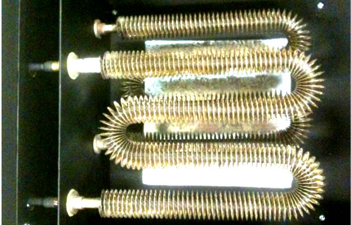
Figure 3.5 Photograph of the W-shaped finrod tubular heater assembly.
