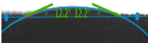
Figure E. 8: Lowest contact angle obtained with the synthesized solution of 750ppm MES + 250ppm CaCl 2 + alkaline condition (Buff Berea)
