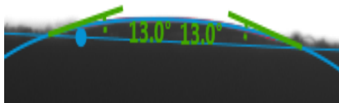
Figure E. 7: Lowest contact angle obtained with the synthesized solution of 750ppm MES + 250ppm CaCl 2 + alkaline condition (Grey Berea)
