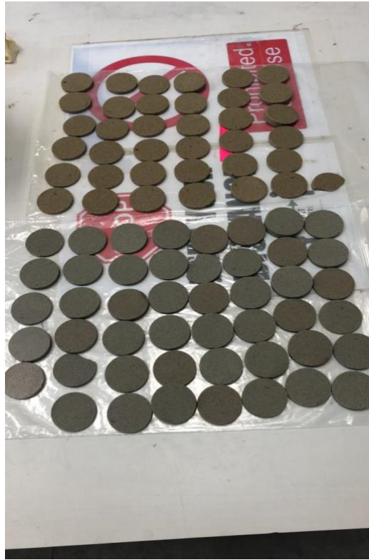
Figure E. 1: Preparation of rock samples (sliced and grinded)
