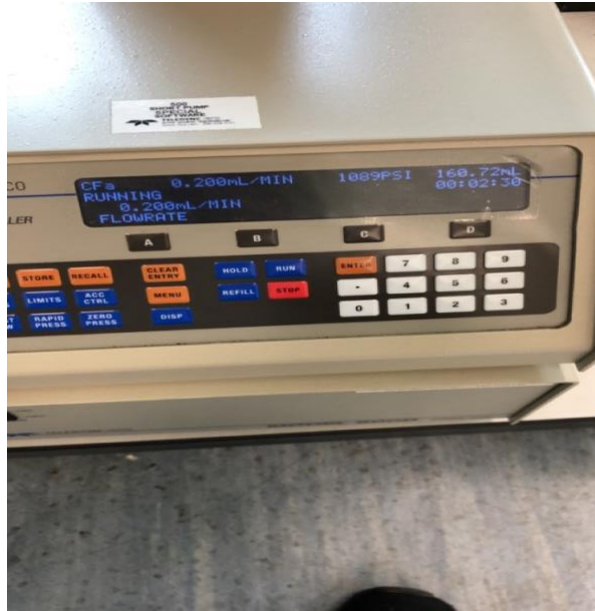
Figure E. 5: Pump used for core-flooding test and adjust the flow rates
