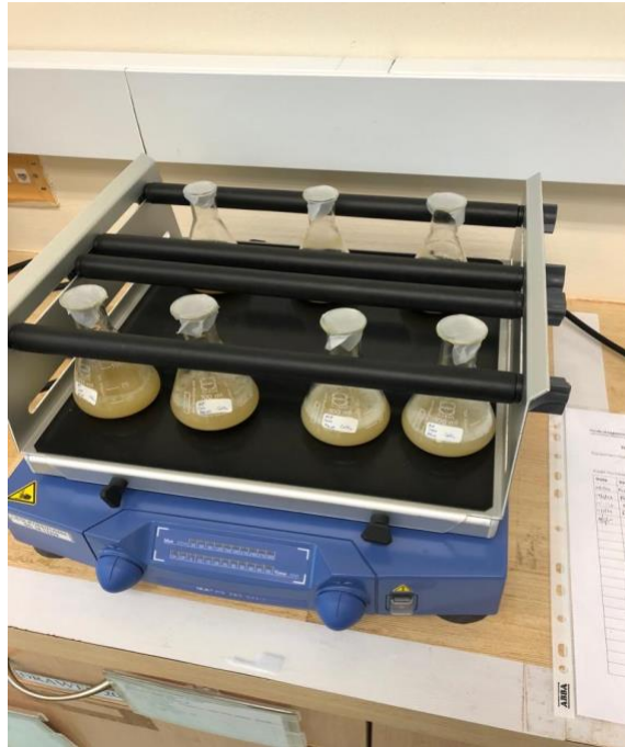
Figure E. 3: Shaking the synthesized solutions with Grey Berea fines (equilibrium process)
