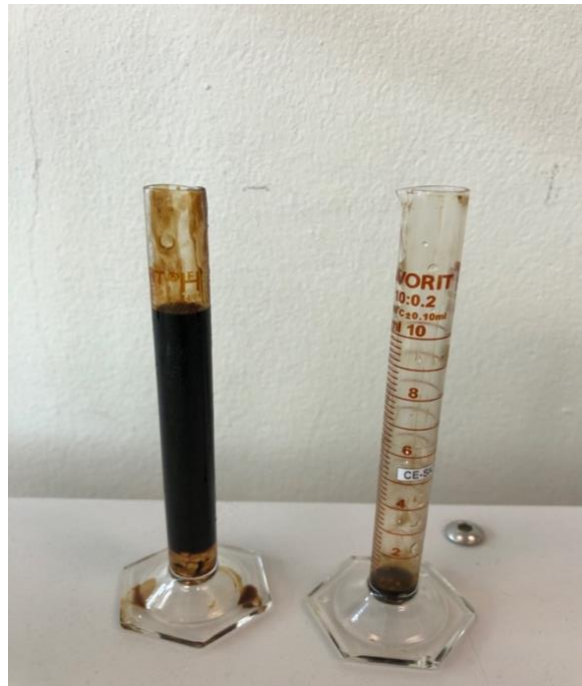
Figure E. 6: Oil recovered during core-flooding test
