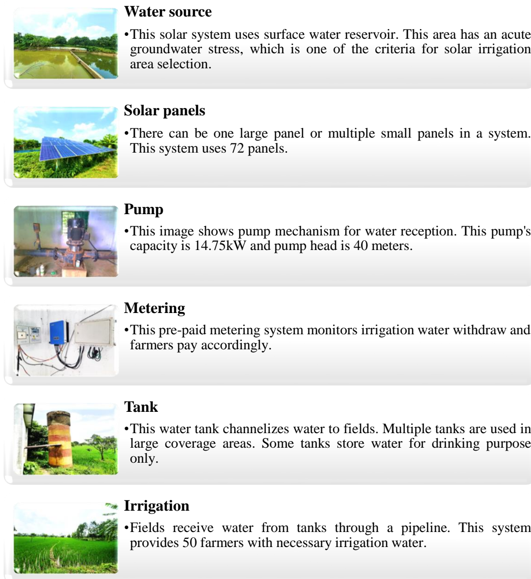
Figure 2. 3 Mechanism of a solar irrigation system in Bangladesh.
