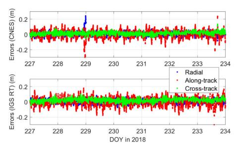
**Figure 5.** Connected orbital errors predicted for 6–11 min for Sentinel-3B from 15 to 21 August 2018. The CNES real-time products (**top**) and IGS RTS products (**bottom**) were used for the processing.
