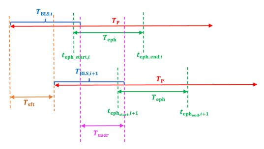
**Figure 2.** Time scheme for real-time LEO satellite POD based on the near-real-time BLS adjustment, the short-term prediction, and the ephemeris fitting.
