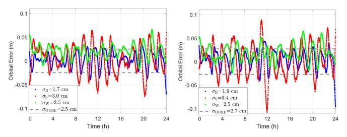
**Figure 3.** Near-real-time BLS orbital errors of Sentinel-3B on 15 August 2018 using (**left**) the CNES real-time products and (**right**) the IGS RTS products.
