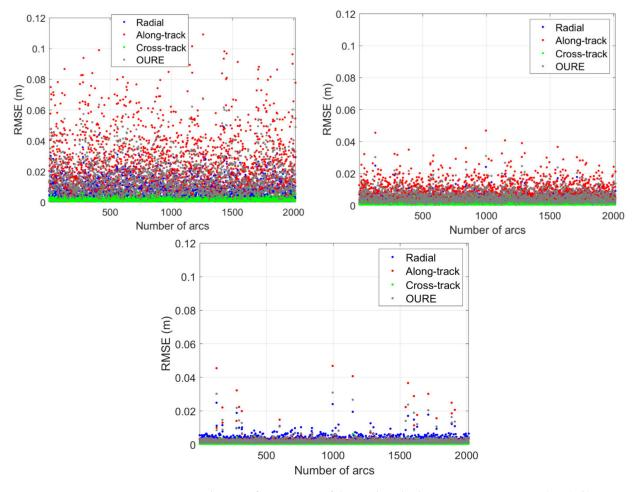
**Figure 7.** Ephemeris fitting errors of the predicted orbits at 5 to 15 min using (**top left**) 16 parameters, (**top right**) 18 parameters, and (**bottom**) 22 parameters. Data from Sentinel-3B and CNES real-time GNSS products from 15 to 21 August 2018 were used for the plots.
