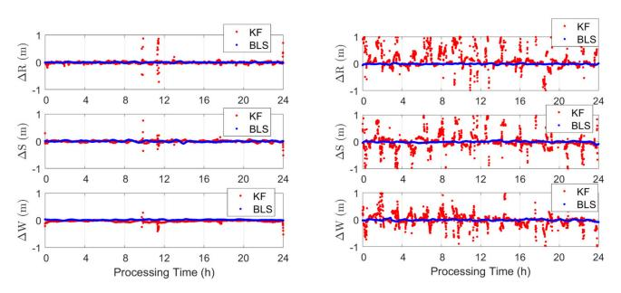
**Figure 1.** Orbital errors processed with the Kalman Filter (KF) in real-time and the Batch Least-Squares (BLS) adjustment in near-real-time. The data of GRACE C on 14 August 2018 (**left**) and 12 August 2022 (**right**) were processed using the CNES real-time GNSS products.
