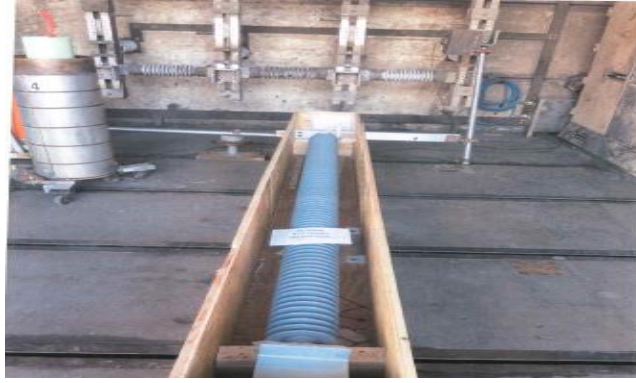
Fig. 5.18. 132-kV NCIT set up for experiment.
