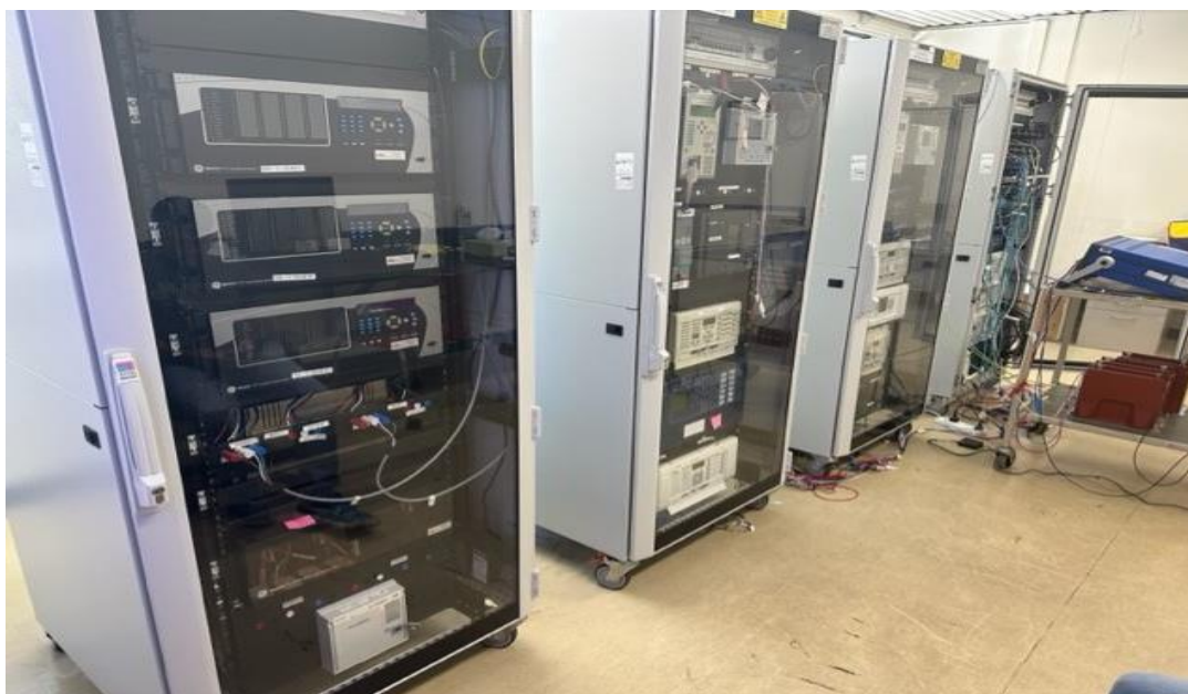
Fig. 7.6. Virtual SAS Network with Smart Technology and IEDs to Test For Cyberattack.
