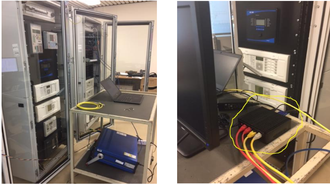
Fig. 4.15. Experimental set-up of the two WAN substation.
