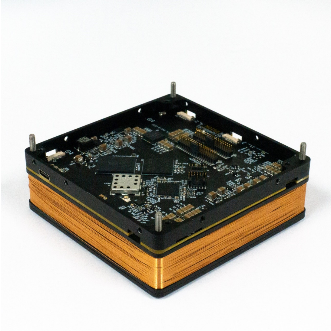
Figure 2.15: The main novel output of the Binar Space Program, the BCC. The external features include the structure and integrated Z-axis magnetorquer. The Binar EPS, ADCS, and flight computer system are inside the core. Testing the functionality of the custom designs was one of the primary objectives of Binar-1.
