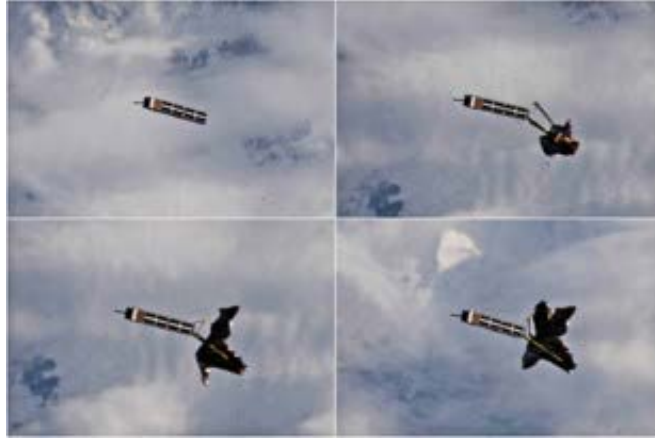
Figure 1.6: The Exo-break technology as pictured after deployment from the ISS on TechEdSat 10. This version of the Exo-break was able to be controlled to manipulate the re-entry location [73]
