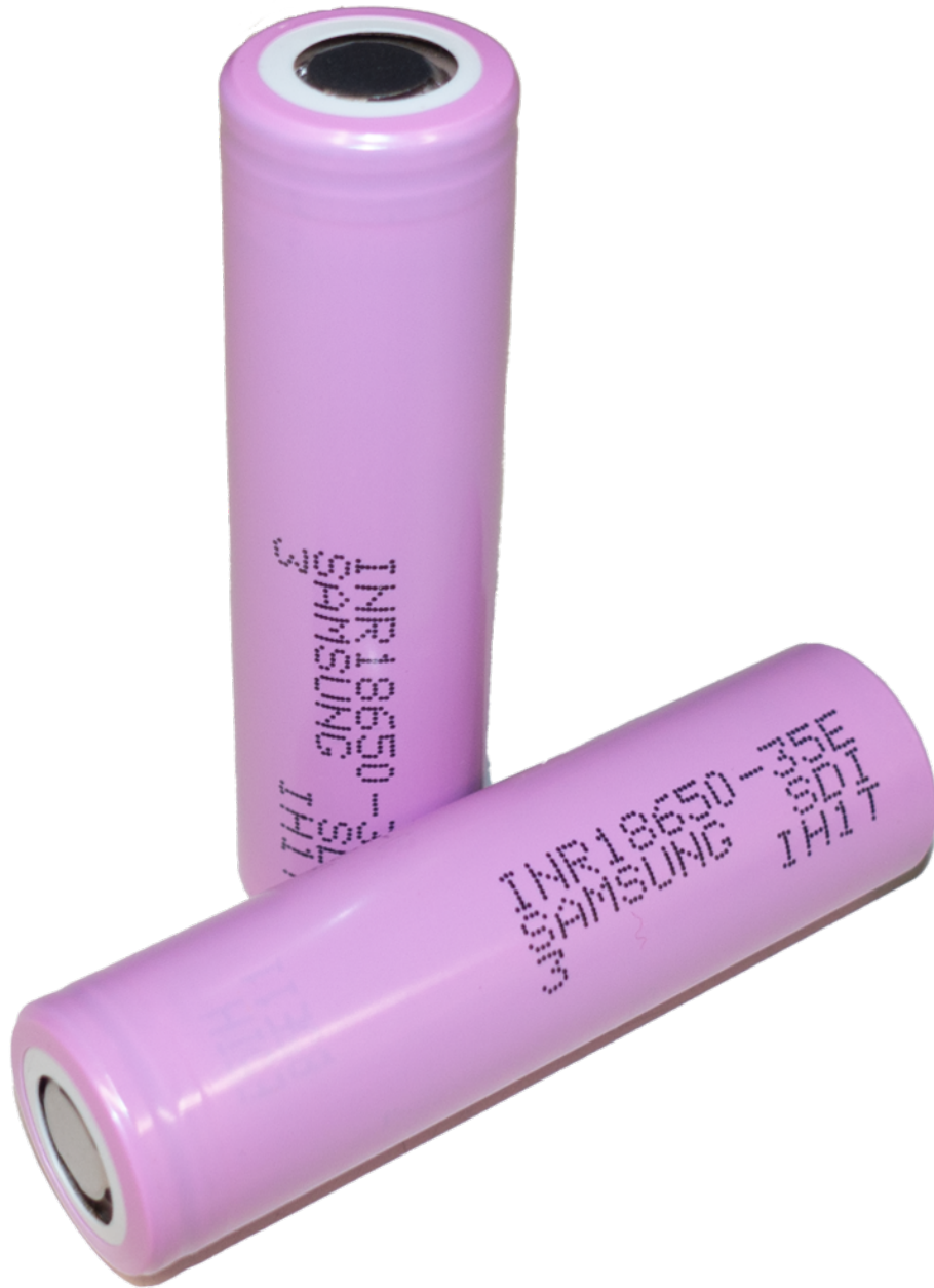
Figure 2.5: The Samsung INR18650-35E lithium-ion battery cell. Each cell has an approximate capacity of 3250mAh and a nominal voltage of 3.7V. When combined into the final 2S2P battery pack, the BCC has a total power storage of 48.1Whr.
