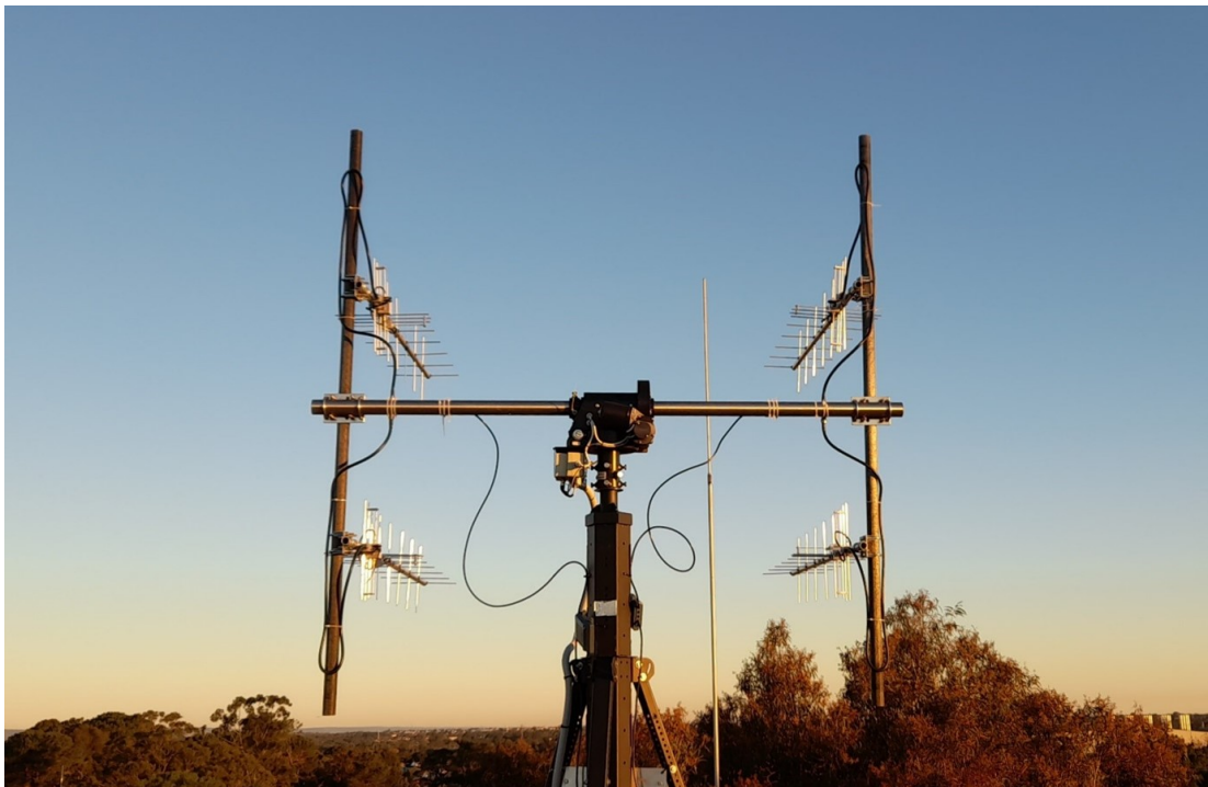
Figure 3.1: The Binar Ground Station antenna pictured above Curtin University in Perth, Western Australia. The complete system will be used in all Binar LEO missions for the foreseeable future and will play an essential role in satellite operations and communications at the university.
