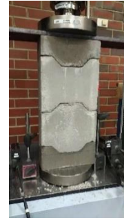
Figure 3-4. Compressive test setup for 2-block prism.
