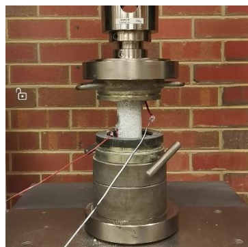
(a) Uniaxial compressive test
