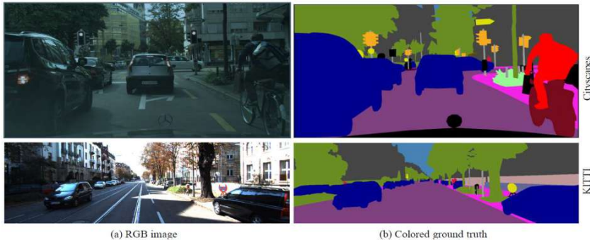
Fig. 1. Pixel labelling in semantic segmentation. First column in the figure shows the RGB images taken from Cityscapes [3] and KITTI [4] data sets and the second column exhibits the corresponding colored ground truth in which pixels from same class are clustered together and received a specific color code based on the class.
