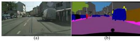
FIGURE 1. Labelling class to each pixel in semantic segmentation. (a) Original input image, (b) colored annotation of the input image where each pixel of the image has a specific color code.
