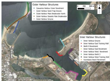
Fig.6. Breakwater structures' locations within the Port of Bunbury. Image source (m p rogers and associates pl, 2020).
