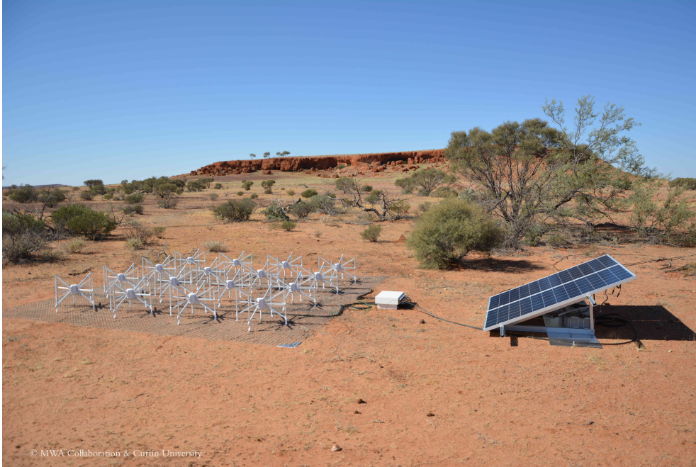
Figure 2.1: A photograph of an MWA tile with a corresponding analog beam-former unit (the ‘white box’) at the MRO site. Each tile consists of 16 equally spaced dual-polarisation dipoles.
