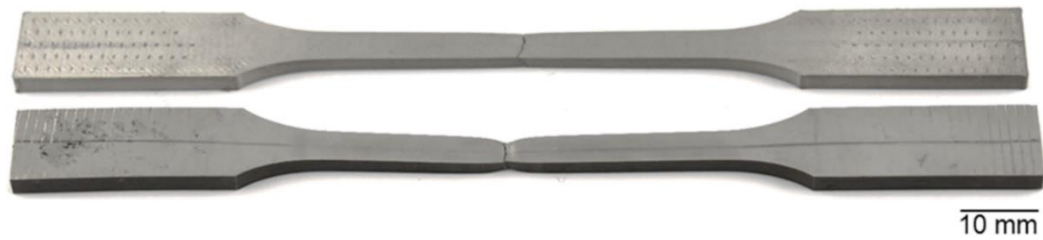
Figure 2-12: Photographic image of both fractured SS316L sintered tensile specimen (top) and SS316L wrought specimen (bottom) showing two types of necked regions
