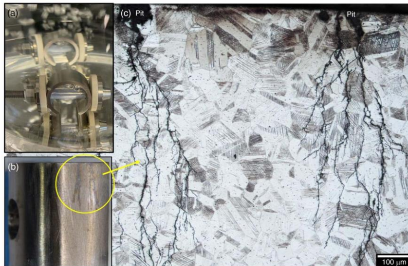
FIGURE 13. CD-wrought SS316L 90% C ring showing (a) full immersion setup, (b) photograph illustrating SCC that started from the edge of the uppermost curved surface, and (c) a micrograph showing the resulting transgranular SCC morphology.
