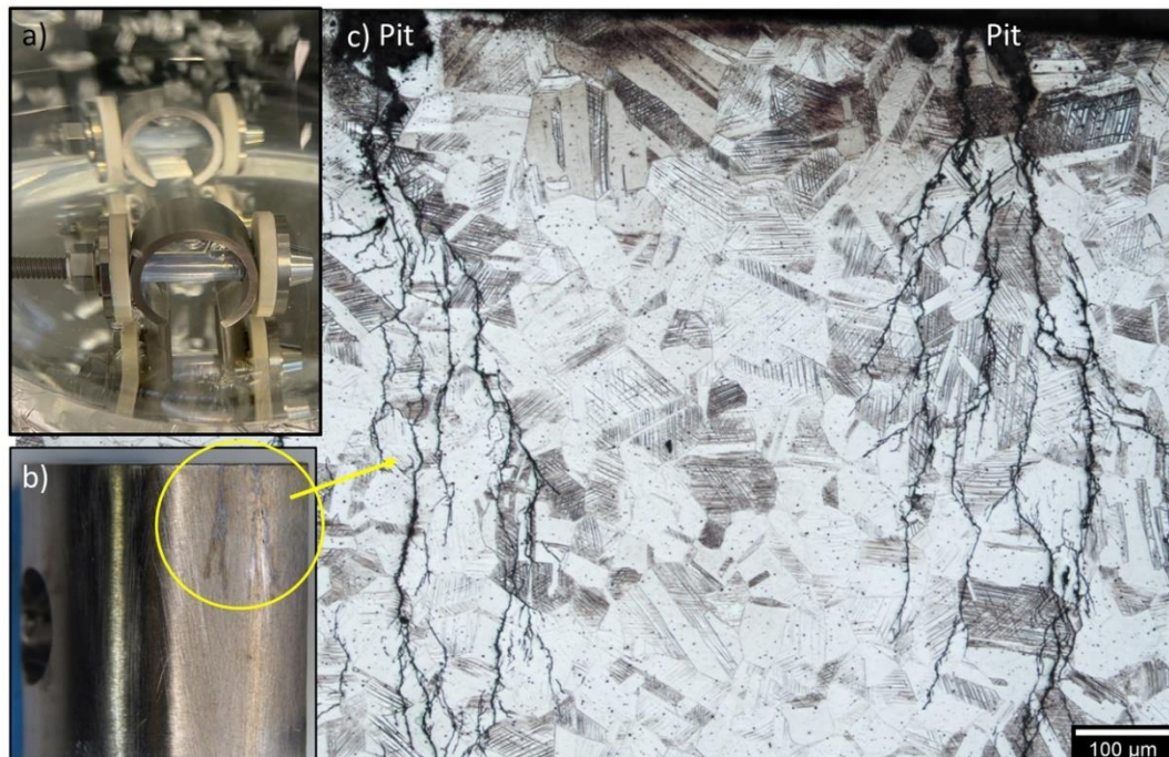
Figure 5-13: CD wrought SS316L 90% C-ring showing a) full immersion setup, b) photograph illustrating SCC that started from the edge of the uppermost curved surface, and c) a micrograph showing the resulting transgranular SCC morphology
