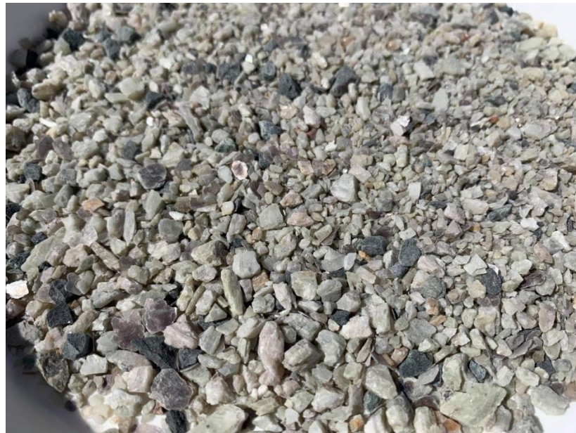
Figure 4-3. Alpha spodumene sample showing coarse size fractions of green spodumene
