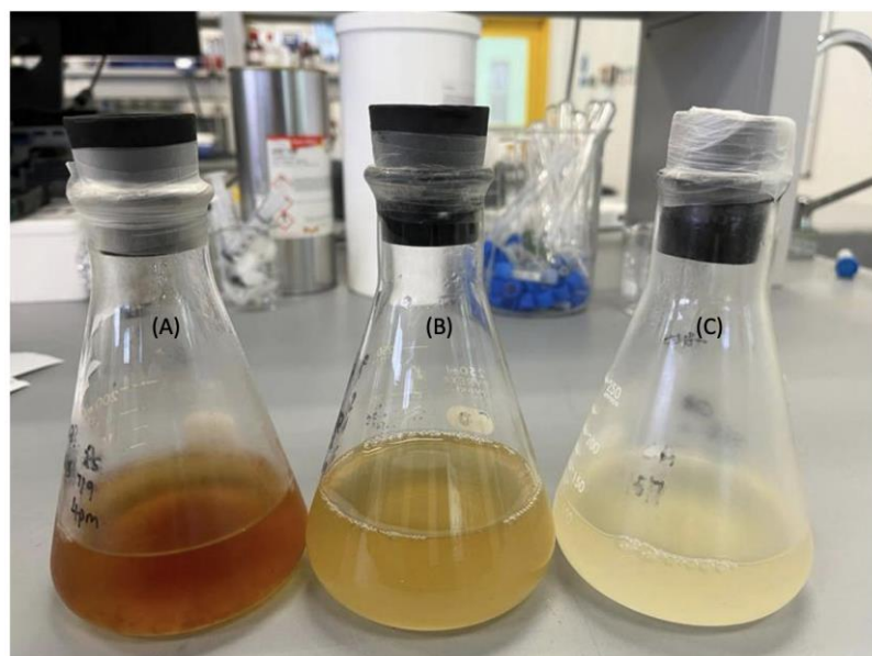
Figure 6.1: Comparison of light (A) and dark (C) fermentation with single stage hybrid fermentation (B).
