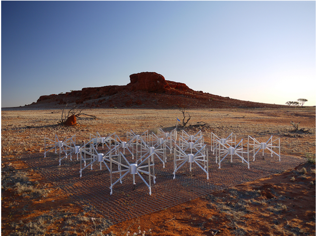
Figure 1.1: Single MWA tile at Inyarrimanha Ilgari Bundara the CSIRO Murchison Radio-astronomy Observatory. Credit: Natasha Hurley-Walker ICRAR/Curtin.
