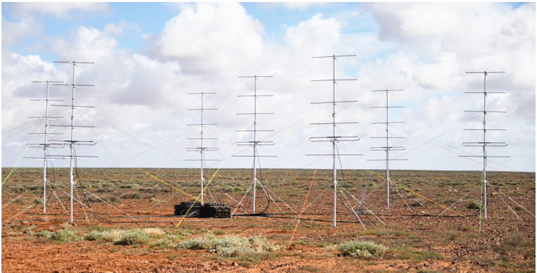
Figure A.2: Sparse array configuration with the antennas directed at Zenith. Array elements configured in a hexagonal configuration with an element separation of \lambda .
