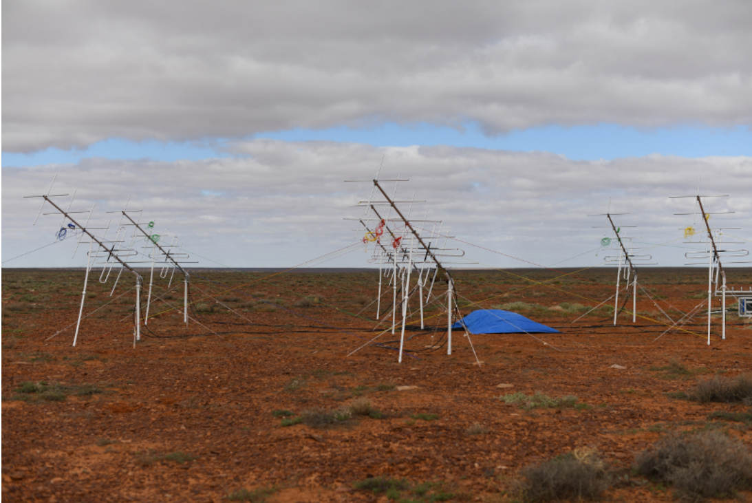
Figure A.3: Hypersparse array configuration with the antennas directed at 30^\circ elevation above the horizon. Array elements configured in a hexagonal configuration with an element separation of 2.5 \lambda .
