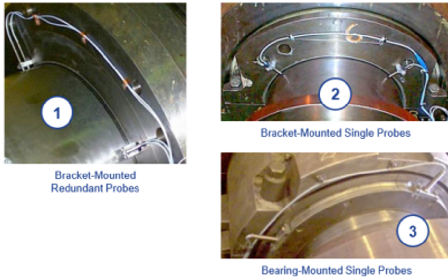
Figure 3.6: Radial vibration probes
