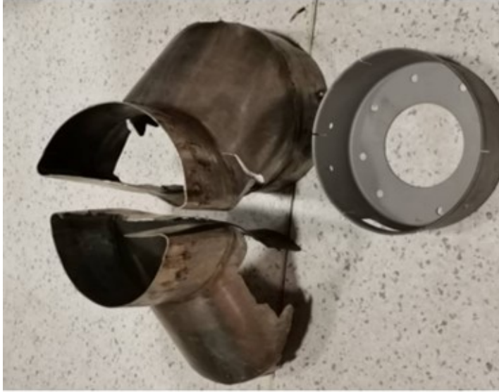
Figure 3.15: Enclosure high temperature due to hot air leaking inside the enclosure
