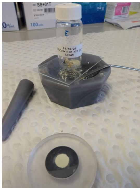
Figure 2-3: Prepared sample for X-ray diffraction in a low background sample holder.
