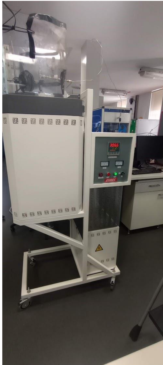
Figure 2-12: Labec VTHTF40/15 high temperature furnace in operation.
