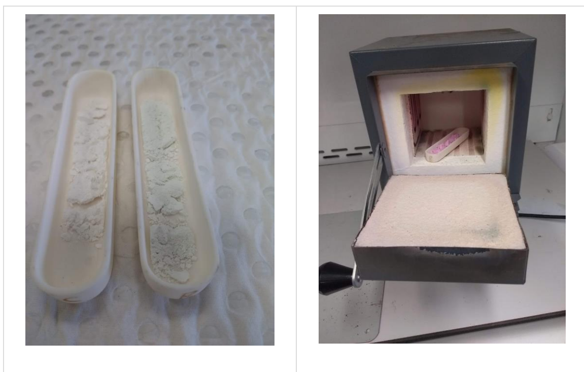
Figure 2-2: Alumina boats used in solid state synthesis (left) FB1310M (ThermoFisher Scientific) furnace used for solid state synthesis (right).
