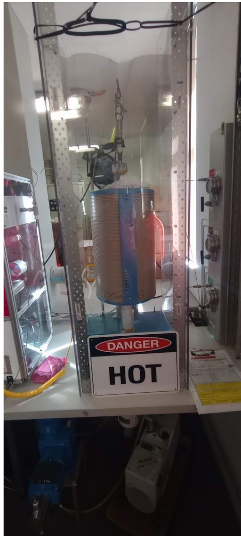
Figure 2-11: Perspex blast shield around the furnace heating the sample cell of the Sieverts apparatus.
