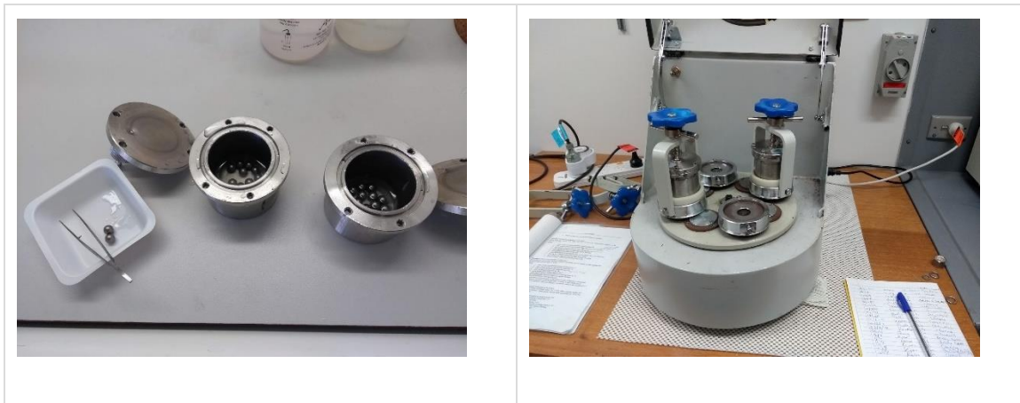
Figure 2-1: Ball milling sample vials with stainless steel balls (left), ball mills loaded for milling.
