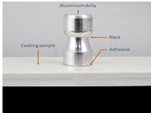
Figure 2-23: Photograph of the dolly attached to a specimen ready for pull-off adhesion tests.
