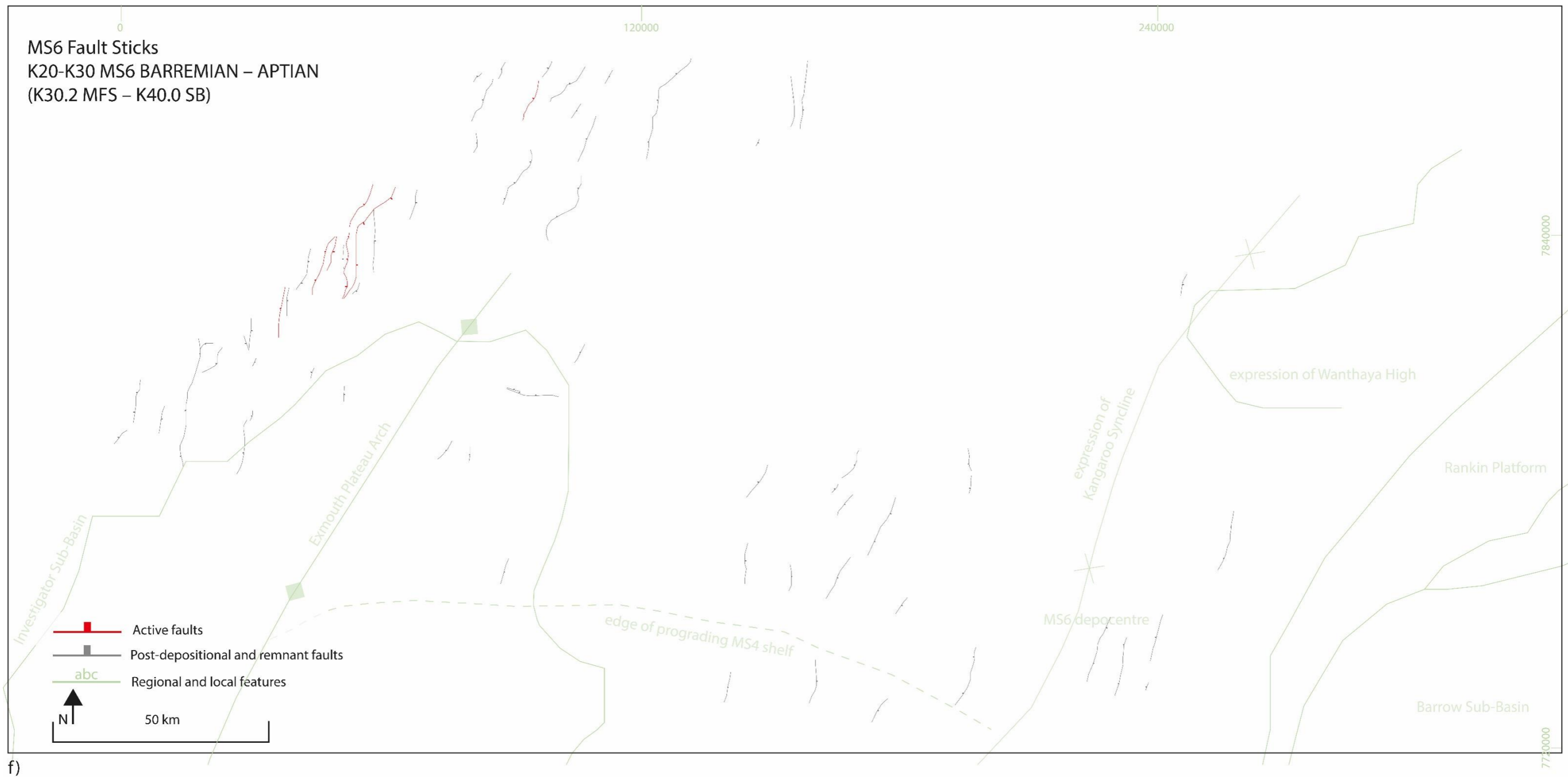
Figure 4.2f Fault stick maps of fault traces as mapped from 3D seismic data. Barremian to mid-Aptian K20-K30 MS6 is intersected by a scattering of faults, where faults largely penetrated the strata after deposition, except in the northwest where some continued movement has been observed. Note that regional scale features are provided in the green underlay, this includes the expression of some features during time frame displayed.
