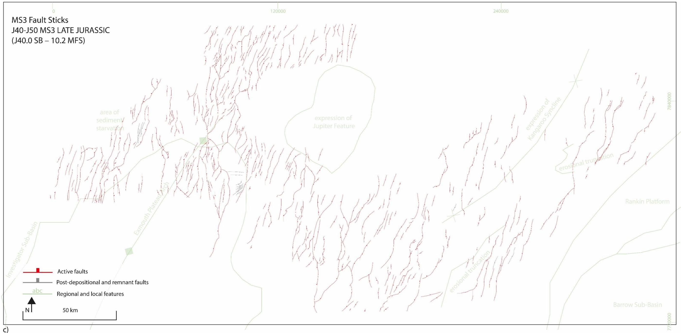
Figure 4.2c Fault stick maps of fault traces as mapped from 3D seismic data. Upper Jurassic to earliest Cretaceous (J40 - K10) age fault activity (red) and faults which penetrate the J40-J50 MS3 stratigraphy following deposition (grey). Fault activity and frequency remains higher in the west of the study area. Note some faults in the east of the study area are now inactive during the deposition of MS3 J50 - K10, after being active for on the deposition of MS2; J20 - J40 (b). Note that regional scale features are provided in the green underlay, this includes the expression of some features during time frame displayed.
