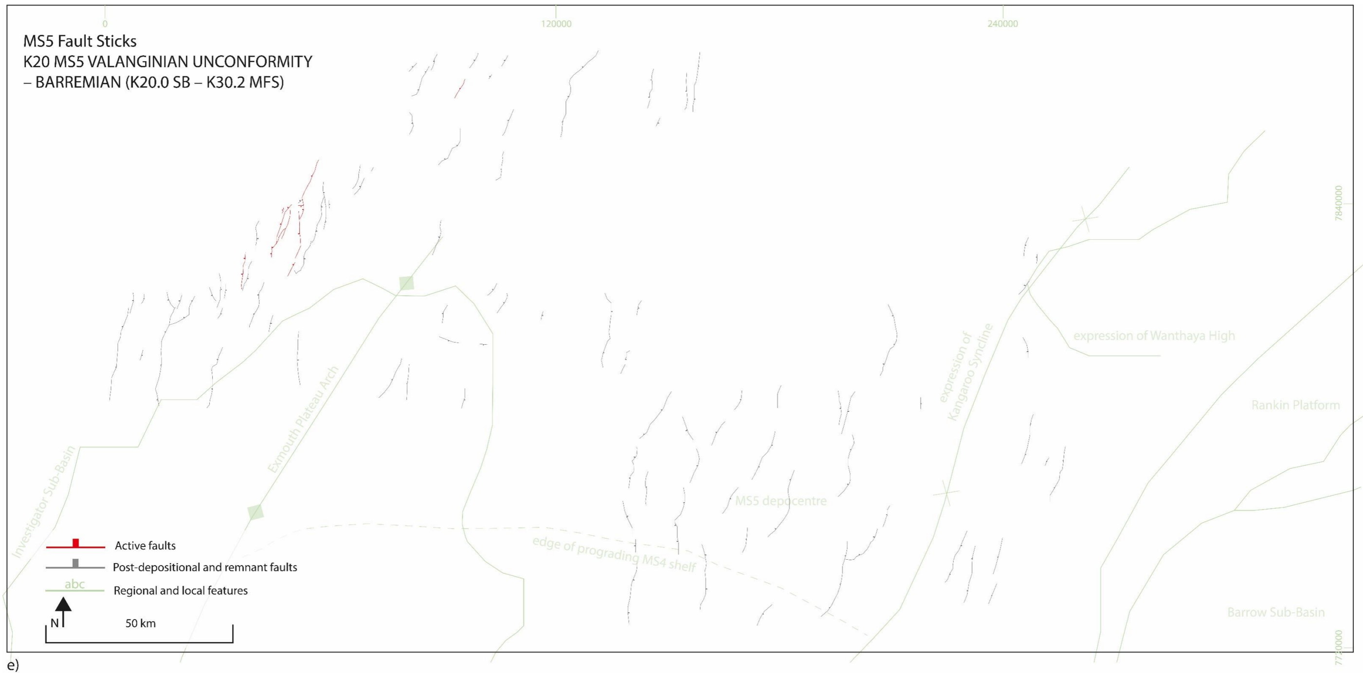
Figure 4.2e Fault stick maps of fault traces as mapped from 3D seismic data. Valanginian (K20, no K10) fault activity is post-depositional penetration of faults through the K20 MS5 strata, with a reduced frequency of faults in the east compared to the west of the study. In the northwest there are a few limited faults where movement is still occurring. Note that regional scale features are provided in the green underlay, this includes the expression of some features during time frame displayed.
