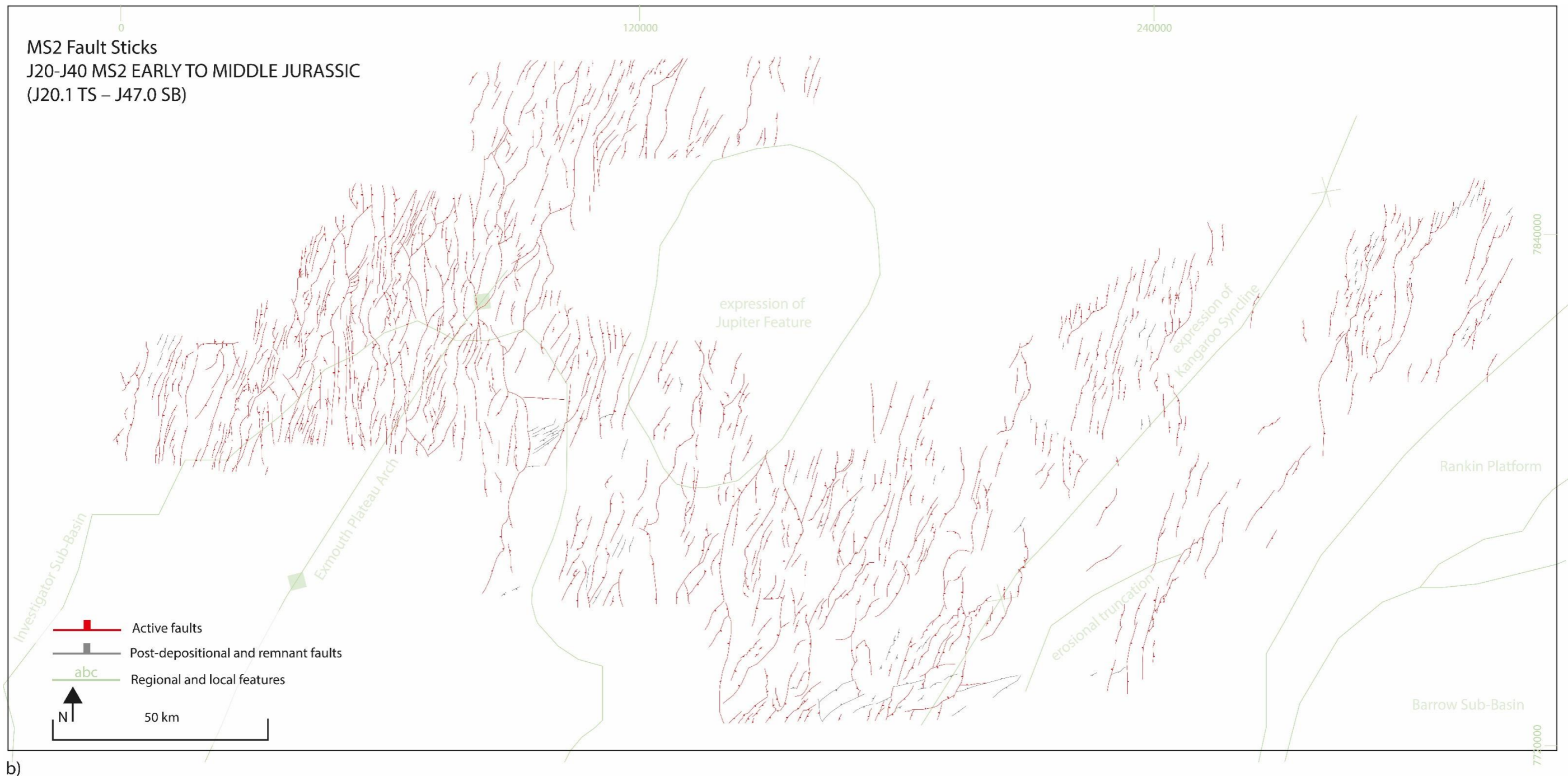
Figure 4.2b Fault stick maps of fault traces as mapped from 3D seismic data. Lower to Middle Jurassic (J20 – J40) fault activity (red) and post-depositional (grey) faults which penetrate the Lower and Middle stratigraphy. The fault sticks showing significant fault activity in the west of the study area, as well as a higher frequency of faults and fault networks in this area. The eastern area of the study area which had limited fault activity during the Rhaetian (TR30) (a) now shows most of the faults to be active. The east to east-north-east orientated faults continues through the strata of the J20-J40 MS2 mega-sequence (Lower and Middle Jurassic). Note the reduced intensity/frequency of fault activity during and following Jurassic deposition in comparison to the a) Rhaetian (TR30) fault activity map. Note that regional scale features are provided in the green underlay, this includes the expression of some features during time period displayed.
