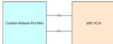
Figure 4. Schematic of the I2C connection between the custom Arduino Pro Mini and the inertial measurement unit. SCL: Serial Clock Line; SDA: Serial Data Line.
