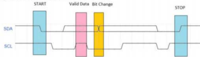
Figure 5. I2C timing diagram. SCL: Serial Clock Line; SDA: Serial Data Line.
