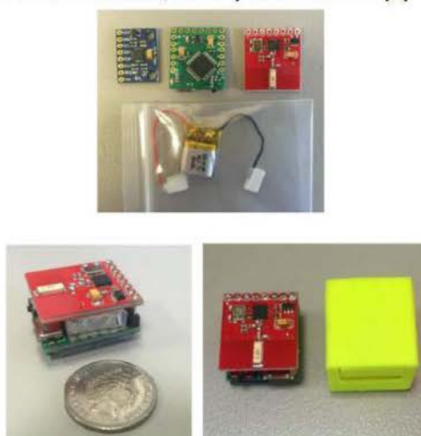
Figure 1. The MPU9150 (blue printed circuit board [PCB]), custom-built Arduino Pro Mini (green PCB), and RF Module (red PCB); a comparison of the inertial measurement unit with an Australian five-cent coin; and the 3D printed case for the sensor [24].
