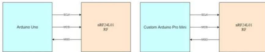
Figure 3. The left diagram shows the serial peripheral interface (SPI) connection between Arduino Uno and the RF module, and the right diagram shows the SPI connection between the custom Arduino Pro mini and the RF module. MISO: Master In Slave Out; MOSI: Master Out Slave In; RF: radio-frequency; SCLK: Serial Clock.
