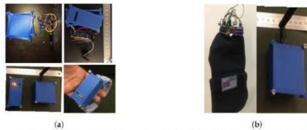
Figure 5. HeadUp system (transmitter and receiver). (a) HeadUp for moderate CP. (b) HeadUp for severe CP.
