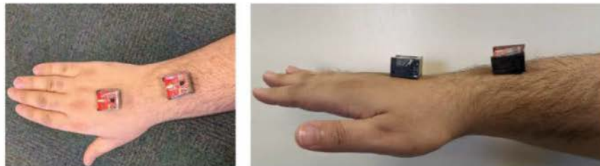
Figure 7. Sensor placement showing sensor 1 connected to the back of the hand and sensor 2 connected above the wrist.
