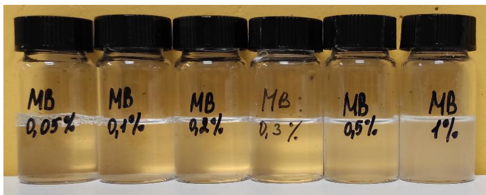
Appearance of surfactant solutions with the addition of sodium metaborate tetrahydrate after 14 days of heating at 70°C
