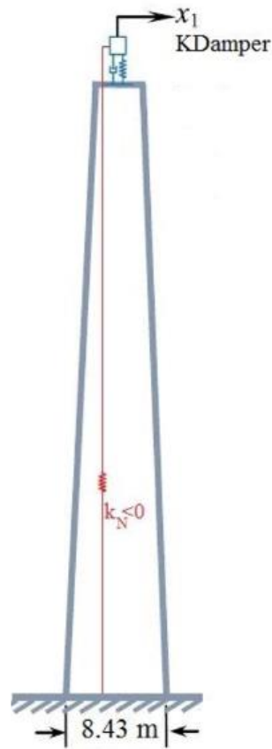
Figure 2-5. The configuration of applying KDamper to a wind turbine model proposed in [55].
