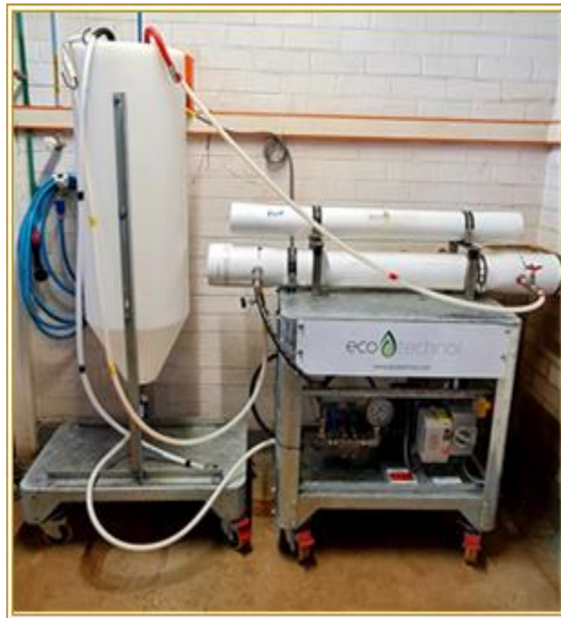
Figure 11 Ultrafiltration / Nanofiltration rig used in this study (Ecotechnol).
