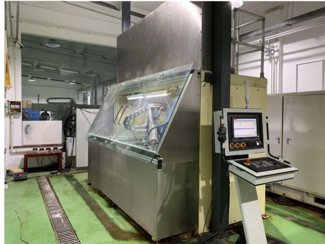
Figure 4. Photograph of the suspension waterjet modification system.
