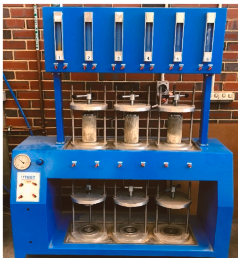
Fig. 6. Water penetration depth test setup.
