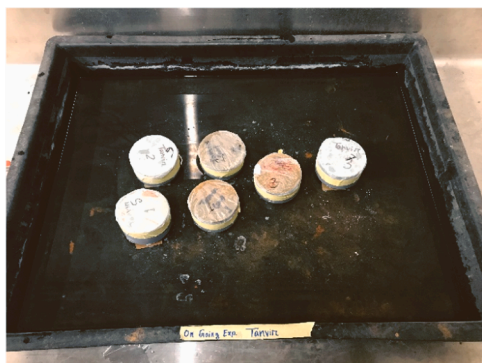
Fig. 5. Sorptivity test of concrete.
