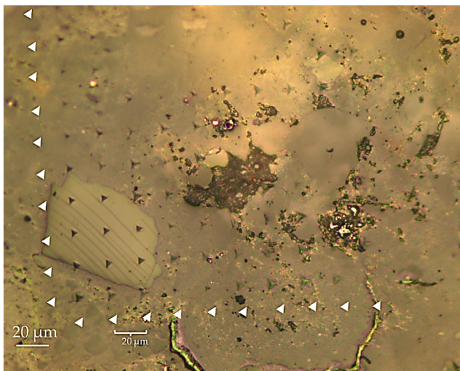
Fig. 4. Typical light microscope micrograph of 200 × 200 μm grid containing impressions of Berkovich indenter on LSG containing 40% silica fume.
