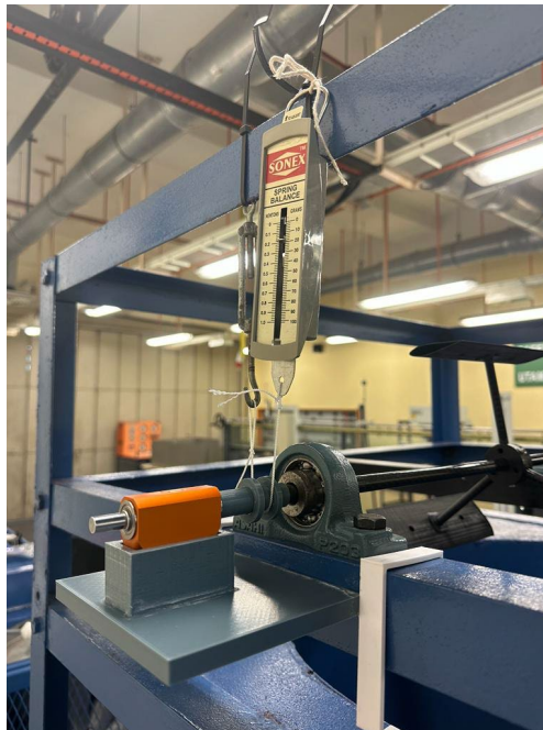
Figure 4.2: Set up of the torque sensor with the pulley.
