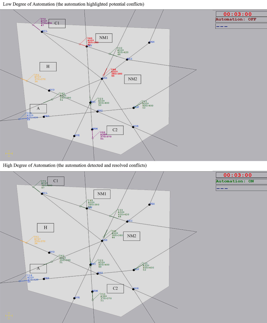
Fig. 3. Sector map of the airspace (labels added to figure for clarity, not presented in-task). Aircraft requiring acceptance (A) and hand-off (H). The box at the top right displays the scenario run-time (red when paused, black when running), and indicates whether the conflict detection automation was active. The top panel shows the low DOA highlighting aircraft pairs at the same altitude. The bottom panel shows the same example with high DOA, where aircraft were not highlighted and conflicts were automatically resolved. The low DOA (upper panel) highlighted all aircraft flying on intersecting flight paths at the same flight level, which includes both conflicts (C1 & C2), and near-misses (NM1 & NM2). The high DOA (lower panel) automatically resolved conflicts (C1 & C2) by allocating one aircraft in the conflict pair to a new altitude (C1 has ascended to 38,000 feet). (For interpretation of the references to colour in this figure legend, the reader is referred to the Web version of this article.)
