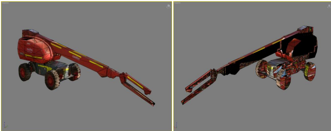
Figure 30. The above images show two sides of the EWP model created using VideoTrace. Areas which were lacking video footage were unable to be modelled.
