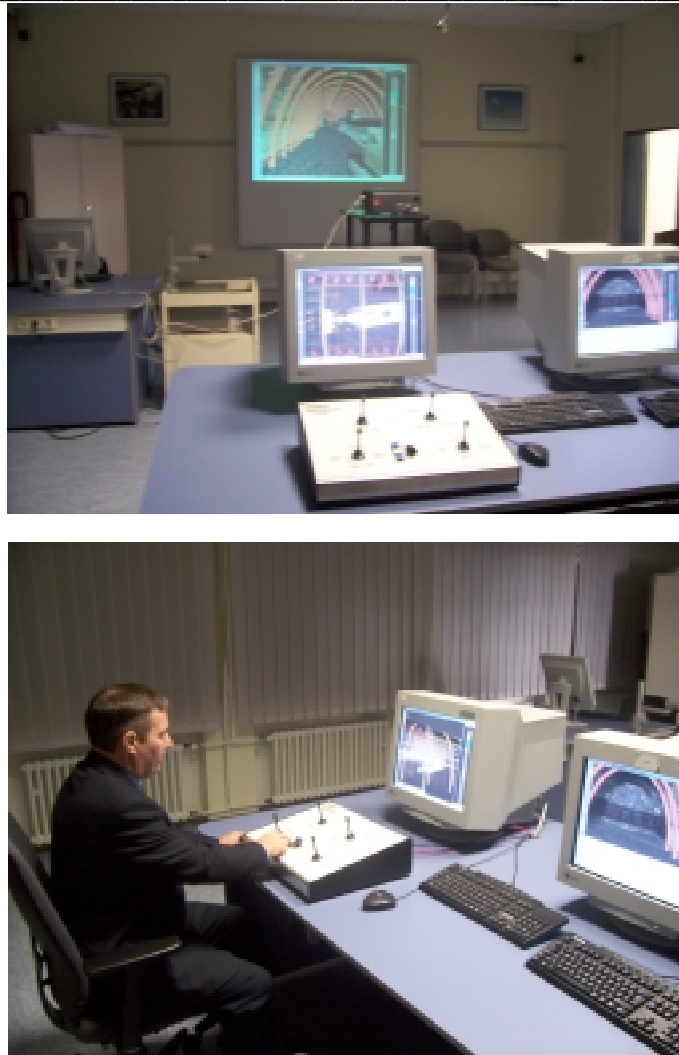
Figure 13. Real machine controls interfaced to the simulation.
