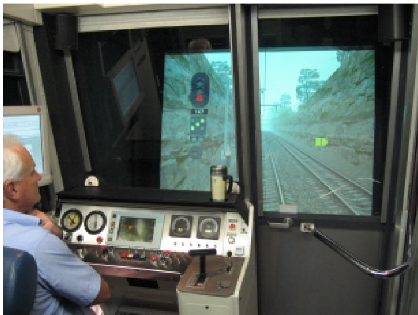
Figure16. Example of RailCorp's Locomotive Training Simulator
