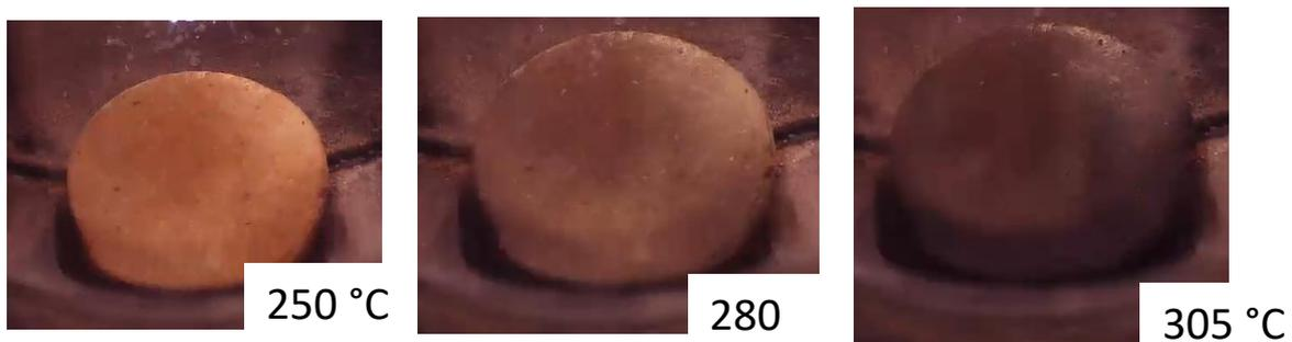
**Figure A6c.** Temperature Programmed Photographic Analysis (TPPA) of  $K_2B_{11}H_{11}Pb$  at a heating rate  $5\text{ }^\circ\text{C min}^{-1}$  under an argon atmosphere
